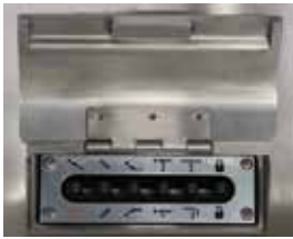
Back-up controls for emergency situations
