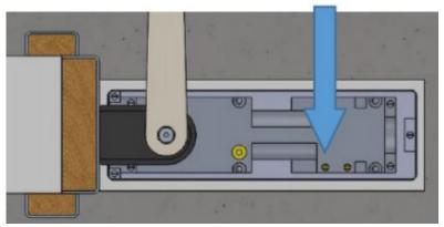
14. . Mark the Location of the closer on the closer body then remove the closer arm. This mark is needed later when the arm is re-fitted.
