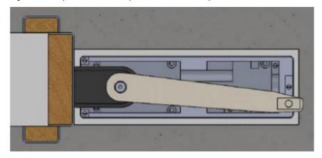
13. Open the arm to roughly 90° in the direction the door will open, this will require a lot of force. Lock the arm in place by carefully, slowly, tightening the 180° - 15° screw fully clockwise. DO NOT USE AN ELECTRIC DRIVER.
