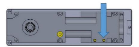
4. 1. Unscrew the closing speed screw until the door begins to close. Keep unscrewing until the desired closing speed is achieved. This should be adjusted at 1/8 turn at a time. Do not fully unscrew this as the closer will be rendered inoperable permanently.
