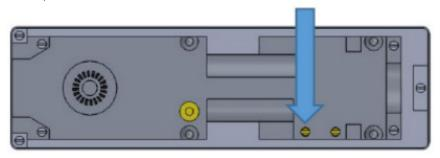
3. . Tighten 0° - 15° [Latching speed] screw until it begins to tighten.
