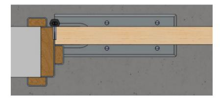
When our recommended frame arrangement is used, the door will open to around 150°. If the full 180° movement the hinge is desired, some of the frame liner, arc and possibly wall needs to cut away at ground level. The cut out will vary between door sets but as a guide 30mm in from the wall, 70mm in from the hinge leaf and 15mm high, flush with the floor.
