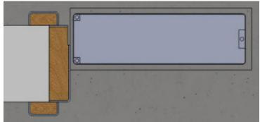
8. Once the housing is located properly, fill the surrounding area with quick drying concrete.
