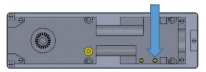
4. Unscrew the closing speed screw until the door begins to close. Keep unscrewing until the desired closing speed is achieved. This should be adjusted at 1/8 turn at a time. Do not fully unscrew this as the closer will be rendered inoperable permanently.
