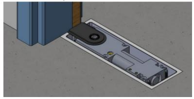
10. Use the 4 adjustment screws to fine tune the closer position, making sure the main body is flush with the floor.
