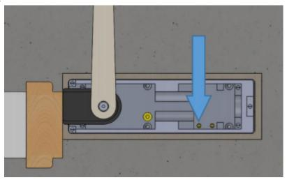
14. Mark the location of the closer arm on the closer body then remove the closer arm. This mark is needed later when the arm is re-fitted.
