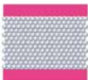
Arrangement of the VACUFORM MicroSpace balls without vacuum
