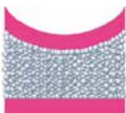
Arrangement of the VACUFORM MicroSpace balls under vacuum
