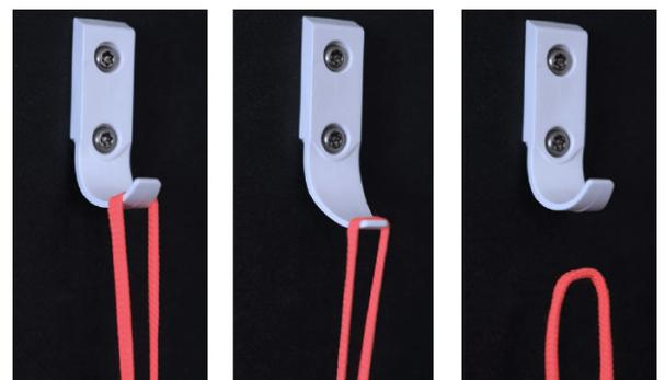
The hook does not break but bends, forcing the ligature to slide off. The hook retains shape and function.
