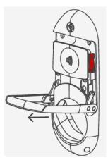
4. Use the emergency lever to pull the door open.
