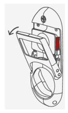
Once the handle has been released, push it down to a horizontal position to unlock the door.
