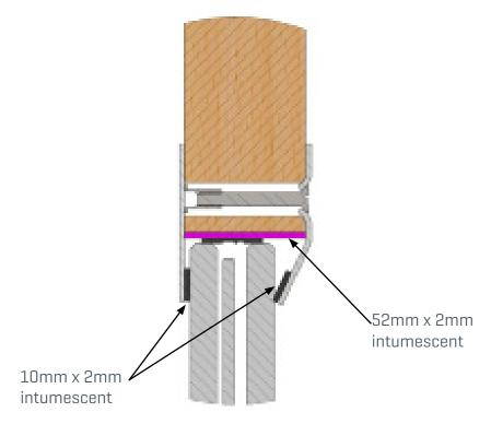
Note: Flat plate goes to the bedroom and the chamfered side goes to the corridor.
