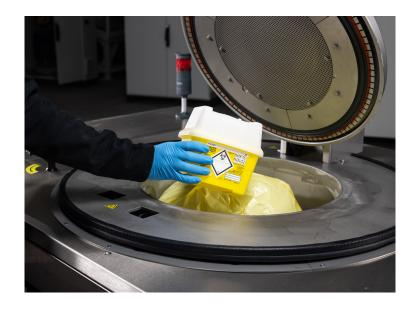
The name Sterilwave® perfectly captures its function: "steril" signifies sterilisation or disinfection, while "wave" represents the microwave technology employed. By grinding up the waste, the volume is reduced by approximately 40 percent. "This reduction means a significant decrease in the number of barrels incinerated annually" says Edwin van Stralen, the team leader of internal logistics and waste management at UMC Utrecht.
