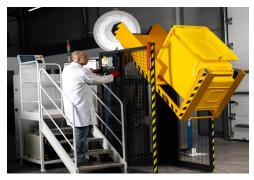
The Sterilwave 900 is the latest solution for highvolumes of biomedical waste. With treatment capacity of 180kg per hour, this unit is designed for large and high-volume facilities.
