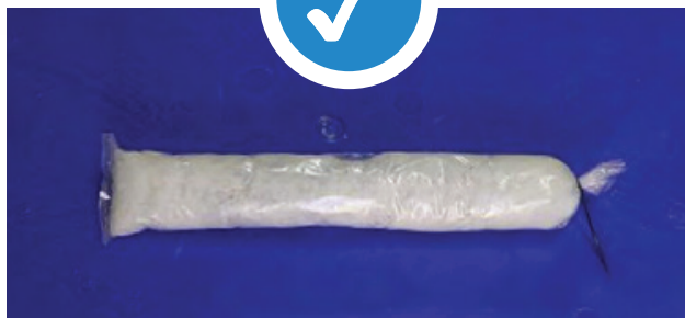
A sealed plastic sleeve that's produced from processing nappies through Incopro. (Contains approx. 30 Adult nappies or 60 child nappies) The bag takes 15 cycles of output before capacity
