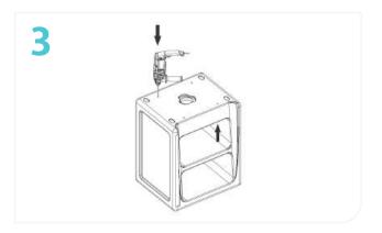
3. Using an extra length 7mm drill bit, drill holes at the marked out points until the drill bit protrudes from the underside of the shelf indicated above.
