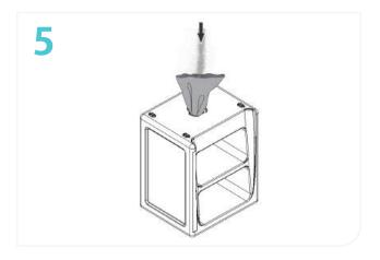
5. Fill the polypropylene bag with the 20kg of sand. Once filled, tie the end of the bag off with a heavy duty cable tie.
