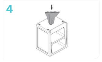
4. Insert the empty polypropylene bag into the cavity of the base of the cabinet. Allow a portion of the bag to protrude from the hole so that a "funnel" is created.
