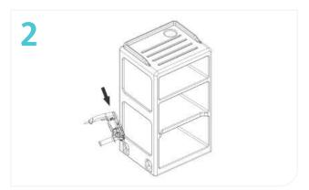
Using the 8mm drill bit, drill through the base of the cabinet in the indicated recesses and into the floor.
