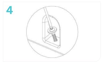
4. Insert the M6 x 60mm Torx screws into the drilled holes and use a Torx security screw driver to tighten all the fasteners making sure the fasteners are flush with the cabinet base.
