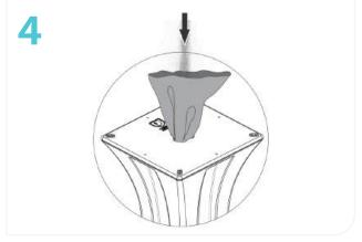
4. Fill the polypropylene bag with the 80kg of sand. Once filled, tie the end of the bag off with a heavy duty cable tie.
