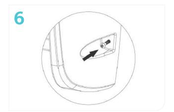
6. Insert the M6 Torx screw into each ofthe holes and tighten using a Torx screw driver. Make sure the shelf is secure against the wall.
