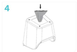
4. Insert the empty polypropylene bag into the cavity of the base of the chair. Allow a portion of the bag to protrude from the hole so that a "funnel" is created.
