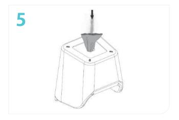
5. Fill the polypropylene bag with the 80kg of sand. Once filled, tie the end of the bag off with a heavy duty cable tie.
