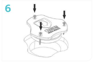
6. Push the bag into the cavity and replace the sand cavity plug. Secure the sand cavity plug into postion with the M4 x 40mm Torx head self tapping screws.
