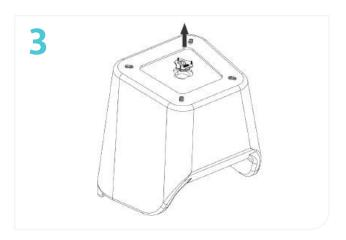
3. Remove the sand cavity plug from the base of the chair.
