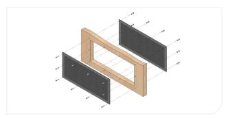
2. Once securely fitted to the door leaf ensure there are no gaps between the grilles and the surface of the door. Any gaps should be filled with anti-pick caulking.
